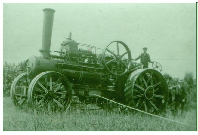
Steam plough, Bill Jarrett driving, Bower Farm, Eynsford, 1920. Freddie Coppins, ploughman by rear wheel. The chain linked to another steam engine on the opposite side of the field and the ploughshare would be pulled across the field from one steam engine to the other
