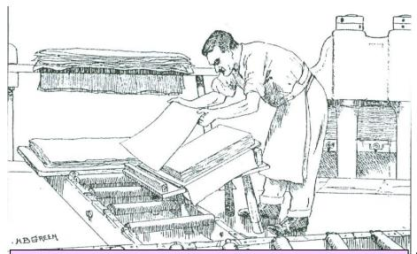
The 'coucher' lays the sheet into a pile, which is then pressed to extract water. The wet paper tears very easily so laying must be done with great care. (The Story of Hand Made Paper, 1924)
